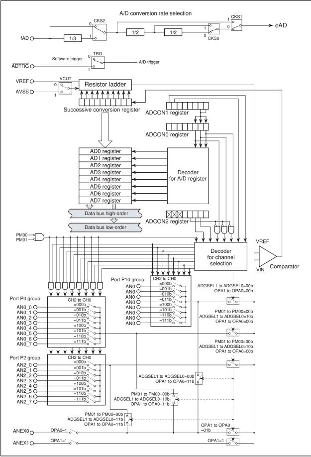
Figure 15.1 A/D Converter Block Diagram
